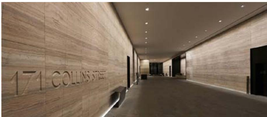
Fig.8 Example of glare control via the usage of backlighting and luminaire shielding (Johnson, 2014)
