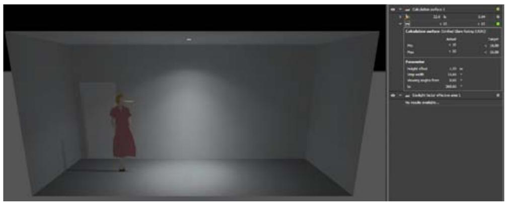
Fig.3 UGR simulation of the brightgreen D700+ CR 55 3K
