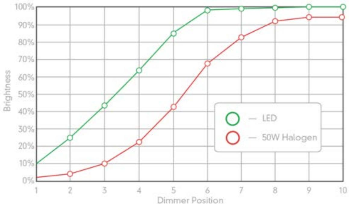
It should also be noted that if LEDs with different transformers are mixed, the dimming of all lights may not track together.
