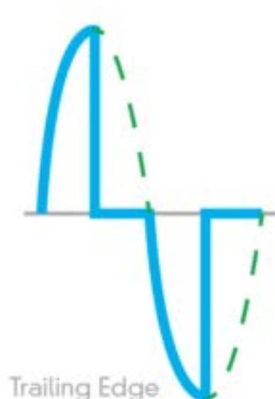
Universal dimming is the newest form of TRIAC dimming. It combines both leading and trailing edge dimming into one module. Universal dimmers have the ability to detect the type of load attached and choose the dimming mode most suited to the load.
