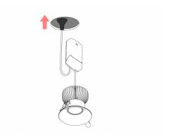
Plug the driver into a mounted general power outlet (GPO) in the ceiling.
